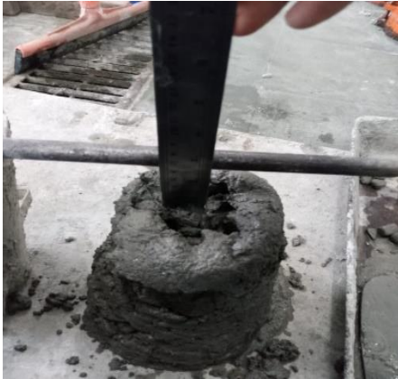
Gambar 1. pengujian slump beton (Sumber: Hasil Penelitian)
